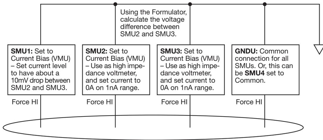
Figure 2. SMU Designation for Four-Point Collinear Probe Measurement
