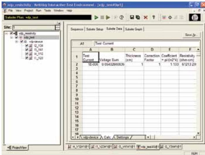
Figure 9. Subsite Data "Calc" Sheet with Resistivity Displayed
