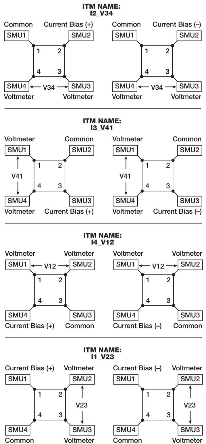
Figure 6. SMU Configurations for van der Pauw Measurements
