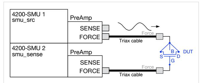
Figure 5. Connection for MOSFET with the gate connected to SMU2 and, with the drain-source-bulk tied together and connected to SMU1 (smu\_sense).
