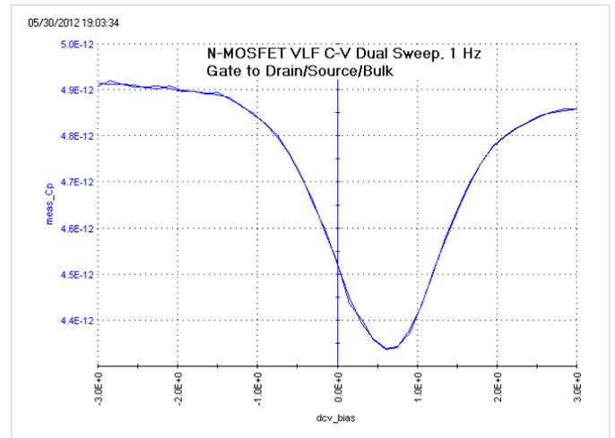
Figure 6. VLF C-V Sweep of an n-MOSFET measured between the gate to drain/source/bulk. This graph is from the *vlf\_nmosfet\_vsweep\_dual* test (user module *vlfcv\_measure\_dual\_sweep\_bias\_fixed\_range*).
