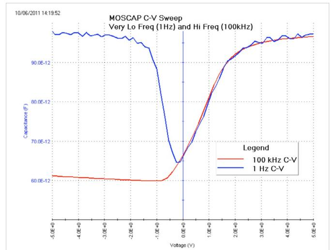
Figure 12. This graph is from the *moscap-vsweep-hif-lof* test, showing the high frequency data from the 4210-CVU card along with the VLF C-V data from the *vlf-moscap-vsweep* test.
