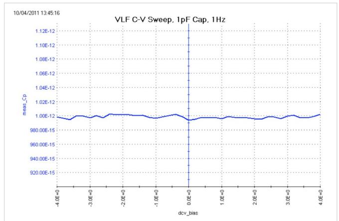
Figure 10. VLF C-V results, at 1Hz, of a voltage sweep on a 1pF reference capacitor. This graph is from the *vlf-cap-vsweep* test (*vlfcv\_measure\_dual\_sweep\_bias\_fixed\_range* user module).
