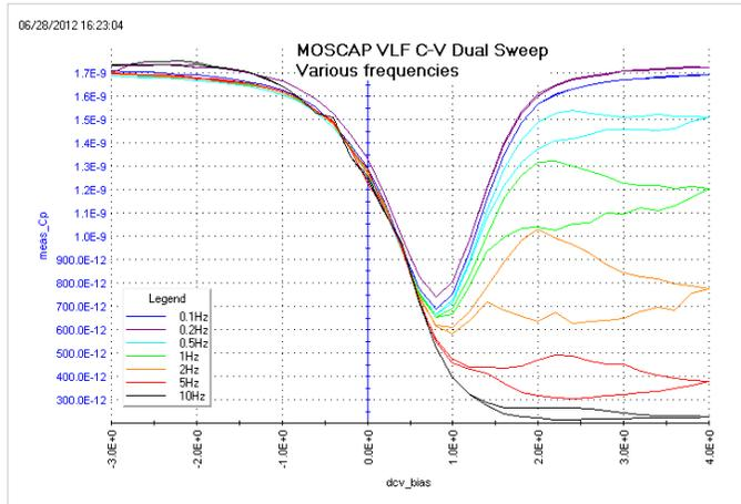
Figure 11. A VLF C-V sweep of a MOSCap at various frequencies from 100mHz to 10Hz created using the *MOS Capacitor VLF-CV Project*. This graph is from the *vlf-moscap-vsweep-dual* test (*vlfcv\_measure\_sweep\_bias\_fixed\_range* user module).
