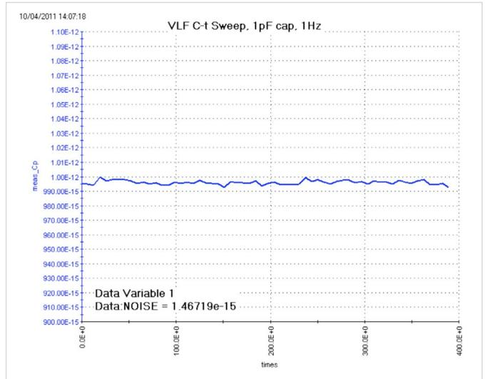
Figure 9. Results of C-t measurements of nominal 1pF reference capacitor, using VLF capacitance technique at a test frequency of 1Hz. This graph is from the *vlf-cap-time* test (user module *vlfcv\_measure\_sweep\_time*).
