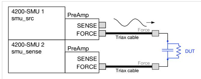
Figure 13. Connection diagram for parallel RC test device.
